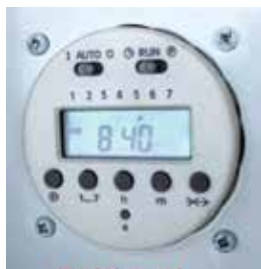
TK-24 DIGITAL SAUNA CONTROL
